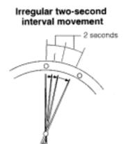
When the watch is again exposed to light after stopping, although the second hand begins to move, since the time is incorrect, the second hand moves irregularly at twosecond intervals to indicate that the time is incorrect. Reset the time after the watch has been sufficiently charged. The second hand will continue to move irregularly at two-second intervals unless the time is reset.
