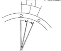
The second hand moves at two-second intervals to indicate that the watch is insufficiently charged. Although the watch will continue to operate normally at this time as well, it will stop after about 2 days have elapsed since the start of twosecond-interval movement. Expose the watch to light to return the second hand to onesecond interval movement.
